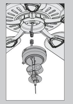
Connect the plugs from the upper and lower switch housings. Make sure to line up the colored markings on the connectors.
